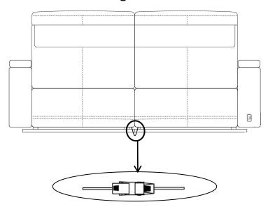
Step8: Plug power parts connection (refer to step 1) into socket at back panel of left hand facing recliner.
