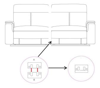
Step7: At the rear and base of lounge, connect the cords between the left hand facing recliner and the right hand facing recliner for electric reclining motion of the left and right recliners.
