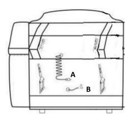
Step6: Connect the right hand facing recliner to the left hand facing recliner. Slide clips together then press the front and rear sides to ensure the clips are connected all the way to the bottom.
